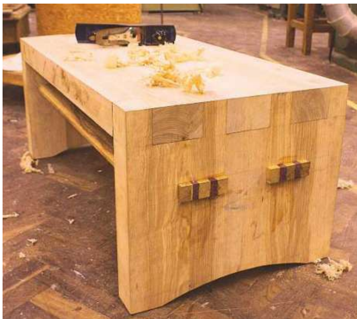
▲ Pic.6 The tenons were left over-size...
